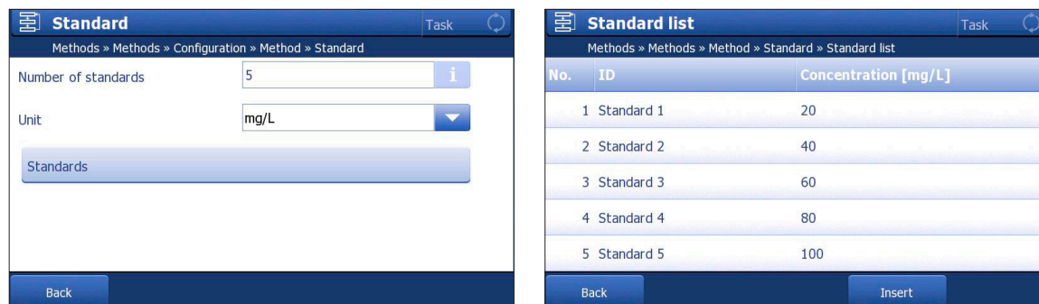
Figure 19: The calibration step and the standard list to determine the calibration line are indicated on the instrument display
